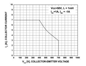
Figure 8. Power Derating Curve
