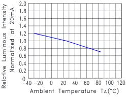
Fig.5 Relative Luminous Intensity VS. Ambient Temperature
