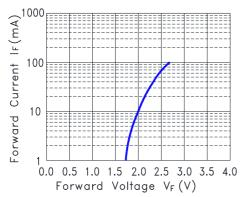
Fig.3 Forward Current vs. Forward Voltage
