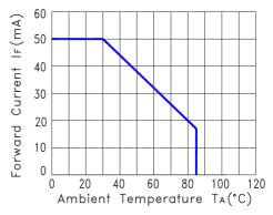
Fig.2 Forward Current Derating Curve
