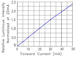
Fig.4 Relative Luminous Intensity vs. Forward Current
