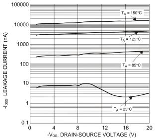
Fig. 9 Typical Drain-Source Leakage Current vs. Voltage
