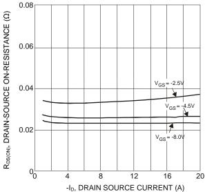
Fig. 3 Typical On-Resistance vs.
