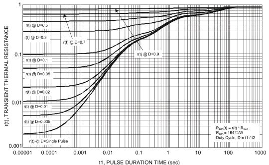
Fig. 12 Transient Thermal Resistance
