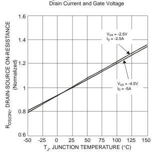
Fig. 5 On-Resistance Variation with Temperature
