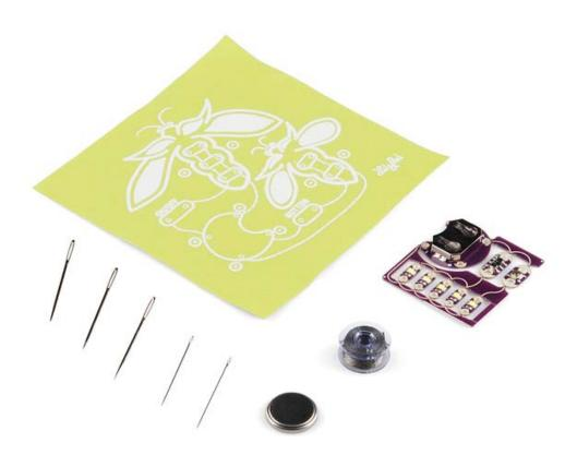
**Description:** The ProtoSnap series is a great way to prototype your project without a breadboard. Everything is wired together on a single board, which makes it easy to explore the possibilities of the components before snapping them apart and building them into your project.
