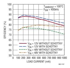
Figure 7. LT8631 Efficiency with/without External Schottky
