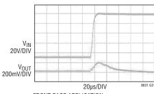
FRONT PAGE APPLICATION 12V to 100V INPUT VOLTAGE TRANSIENT LOAD = 100mA  $C_{OUT} = 2 \times 47 \mu F$
