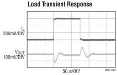
FRONT PAGE APPLICATION 200mA to 800mA LOAD TRANSIENT  $V_{\mbox{\footnotesize{IN}}} = 15 \mbox{\footnotesize{V}}$
