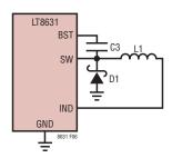
Figure 6. External Schottky Catch Diode
