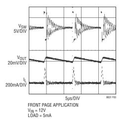
Figure 3. Burst Mode Operation
