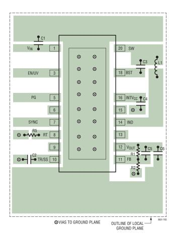
Figure 5. Recommended PCB Layout for the LT8631
