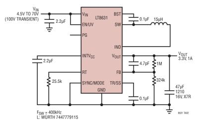
1MHz, 3.3V, 1A Step-Down Converter
