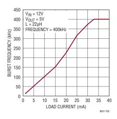
Figure 2. Burst Frequency vs Load Current
