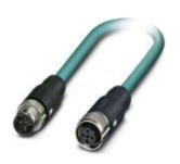
Network cable, Ethernet CAT5 (100 Mbps), Ethernet CAT5e (100 Mbps), 4-position, PUR, water blue RAL 5021, shielded, Plug Straight M12 SPEEDCON / IP67, Coding: D, on Socket Straight M12 SPEEDCON / IP67, Coding: D, Cable length: 1 m
