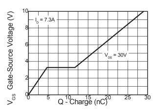
Gate-Source Voltage v Gate Charge
