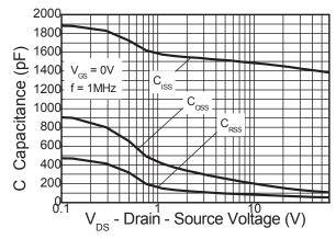
Capacitance v Drain-Source Voltage
