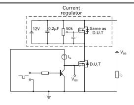
Gate charge test circuit
