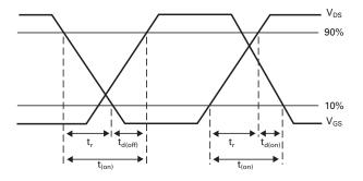
Switching time waveforms
