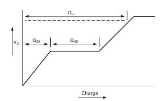
**Basic gate charge waveform**
